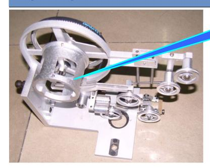
Fixed Axis for accumulating wire spool
